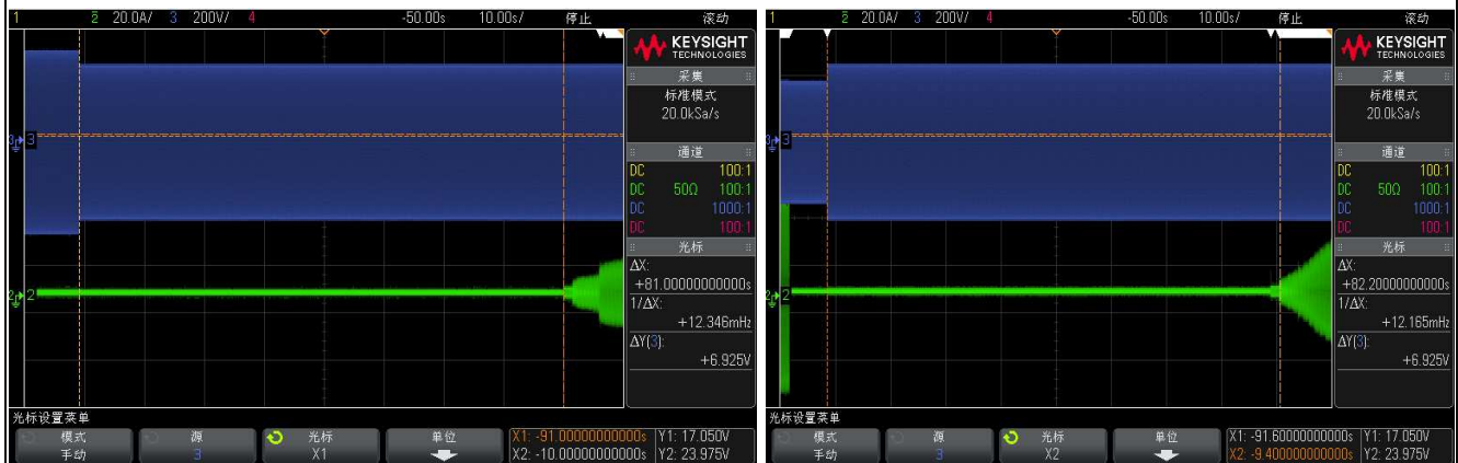
Re-connection after voltage fault
